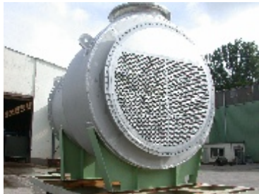
Messrs Ineos Phenol Material= 1.4571 \text{\O} = 2.100 / L = 4.630 / \text{kg} = 21.100
