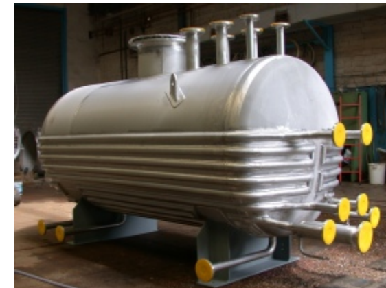
Messrs Bayer Halfpipe \text{\O} 60,3 \times 3 Material= 1.4571 \text{\O} = 1.400 / L = 3.200 / \text{kg} = 1.300
