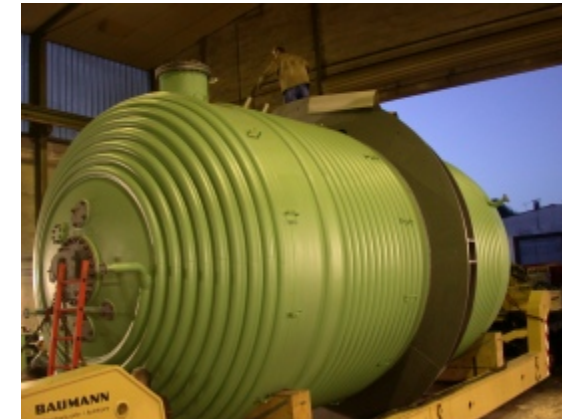
Messrs Tecnimont Distillation vessel w/ halfpipe \text{\O} 60,3 \times 3 Material= P355NH \text{\O} = 4.000 / L = 8.880 / \text{kg} = 32.900
